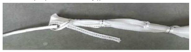
e) Then wrap the inner duct and one end of threading apparatus closely with adhesive tape.
