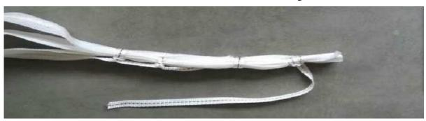
d) Thread the pull tape into one end of threading apparatus and make a fast knot.
