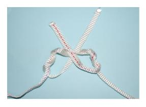
4. then tension the two ends of pull tape to make a knot
